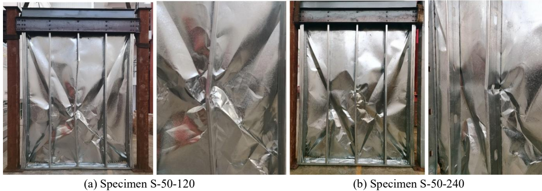
Figure 7. Failure phenomenon of specimen S-50-120 and S-50-240.
