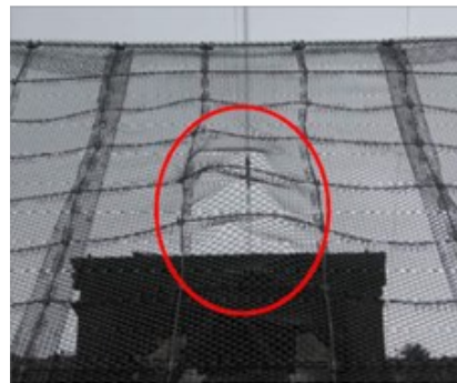
(b) Deformation of wire net after experiment
