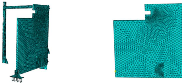
Figure 3. Finite element model of BFRP protective door.
