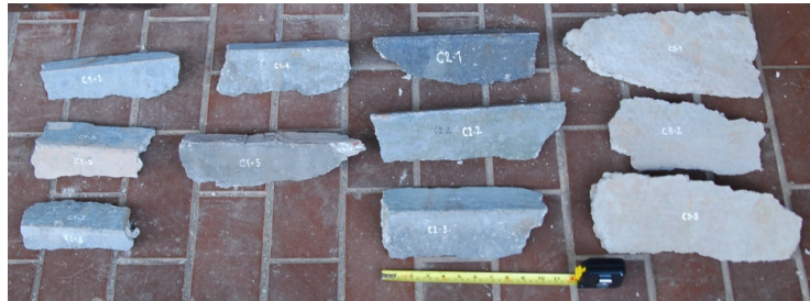
Figure 6. Debris of spalled concrete from tested specimens
