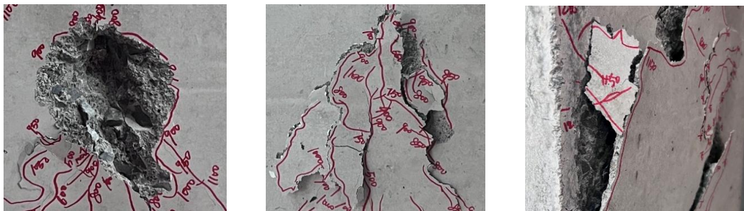
(a) Phenomenon of concrete failure in PZ shear connectors pushed out of specimens
