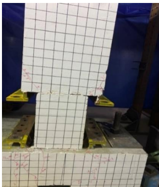
(a) Remove external energy dissipation components of the specimen
