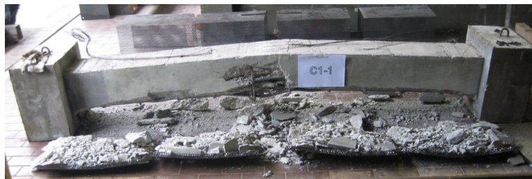
Figure 7. Spalling Image of column specimen C1-1-00 after test
