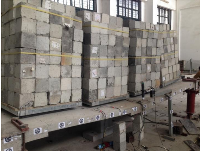
a) A photo of loading process on PC specimen
